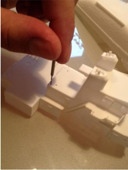
As the parts are printed, some residue (mostly powder) remains in the holes and crevices. Therefore, it is recommended to first clear all holes. This is most easily done with a thin drilling bit of 0.5mm or 1.0mm diameter that is held between two fingers and slightly rotated around each hole. Almost all holes have 1.0mm diameter.
