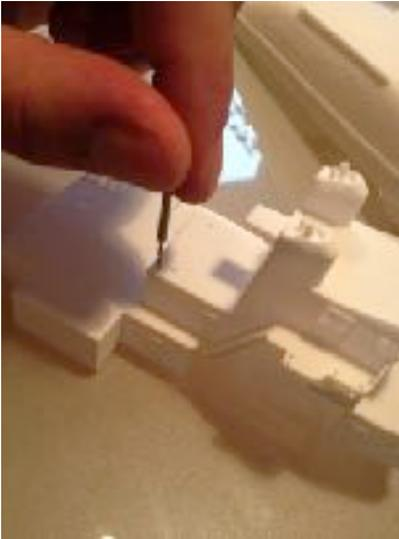
As the parts are printed, some residue (mostly powder) remains in the holes and crevices. Therefore, it is recommended to first clear all holes. This is most easily done with a thin drilling bit of 0.5mm diameter that is held between two fingers and slightly rotated around each hole.
