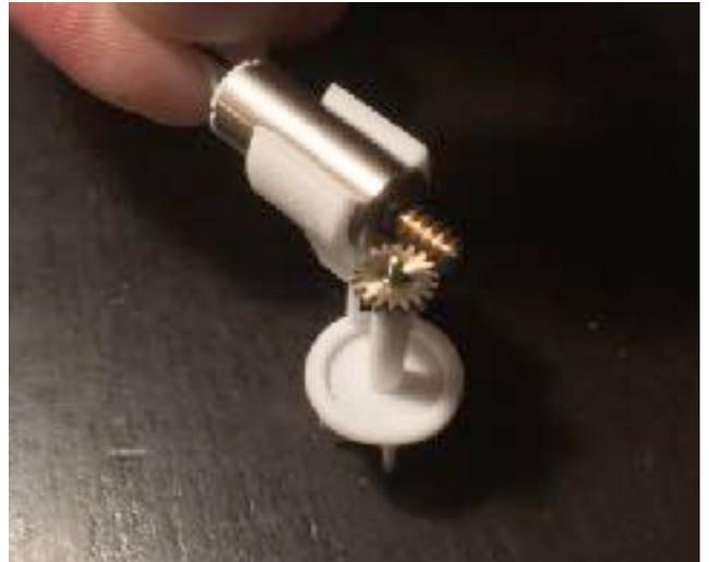
The assembly is rather simple. See the figure below for the sequence of the parts. Make sure you glue the paddle well to the shaft, e.g. with power glue. Also the motor should be fixed in the mount. Usually, the gears can be pushed onto the shafts without much additional glue.
