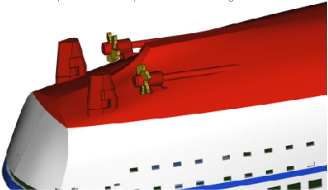
To make the propulsion work, insert the shaft from the back and make sure it aligns with the printed mounts. Typically, you will have to shorten the thread of the shaft to fit the propeller. Use a sharp saw and make sure all parts fit well before gluing them into place.
